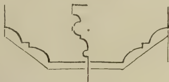
FIG. 1509.—St. Mary's, Auchterhouse. Section of Chancel Arch Mouldings.
